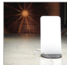
Ecoflex pavement signs tested to Storm Force 10 Beaufort Scale.
